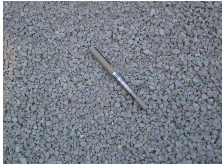
Cured and crushed aggregate
