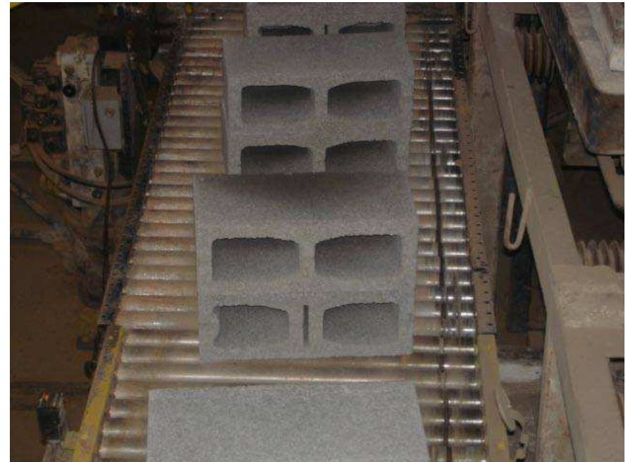
Blocks after curing process
